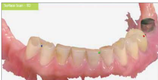
Merging with 3points on the same teeth No. of both data.
